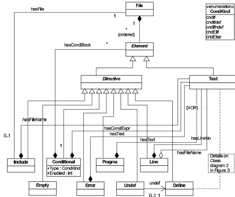
Fig. 2. Schema UML Class diagram - Directive part
