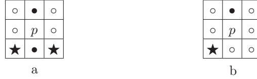
Figure 1: Examples where p is an isolated cavity point (a) and a single border point (b). The positions marked “•”, “★”, and “○” are considered to be active black points, inactive black points, and white points, respectively.
