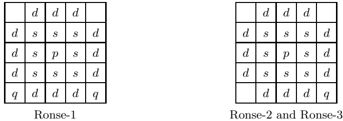
Fig. 4. Local supports of the proposed algorithms. Self-deletability (see Definition 2) of the black point “ p ” is based on points marked “ s ”, double-deletability (see Definition 3) adds points marked “ d ”, and square-deletability (see Definition 4) needs additional points marked “ q ”.
