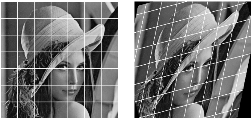
Fig. 2. Example of a 2D affine transformation: The original image (left) and the transformed one (right). Lines are mapped to lines, parallelism is preserved, but angles can be altered
