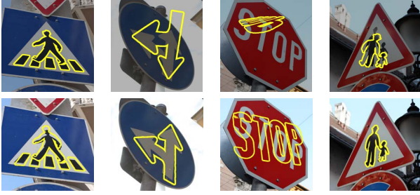
Figure 5. Registration results on traffic signs obtained by SIFT [9]+ homest [8] (first row) and Shape Context [12]+ homest [8] (second row). The contours of the registered images are overlaid.
