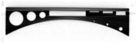
Fig. 16. FBP reconstruction with beam hardening correction for line detector (450 kV, high sampling).
