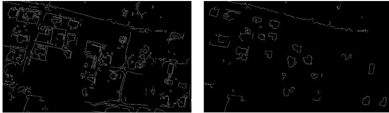
(a) Edge detection on R component (b) Edge detection on u^* component
