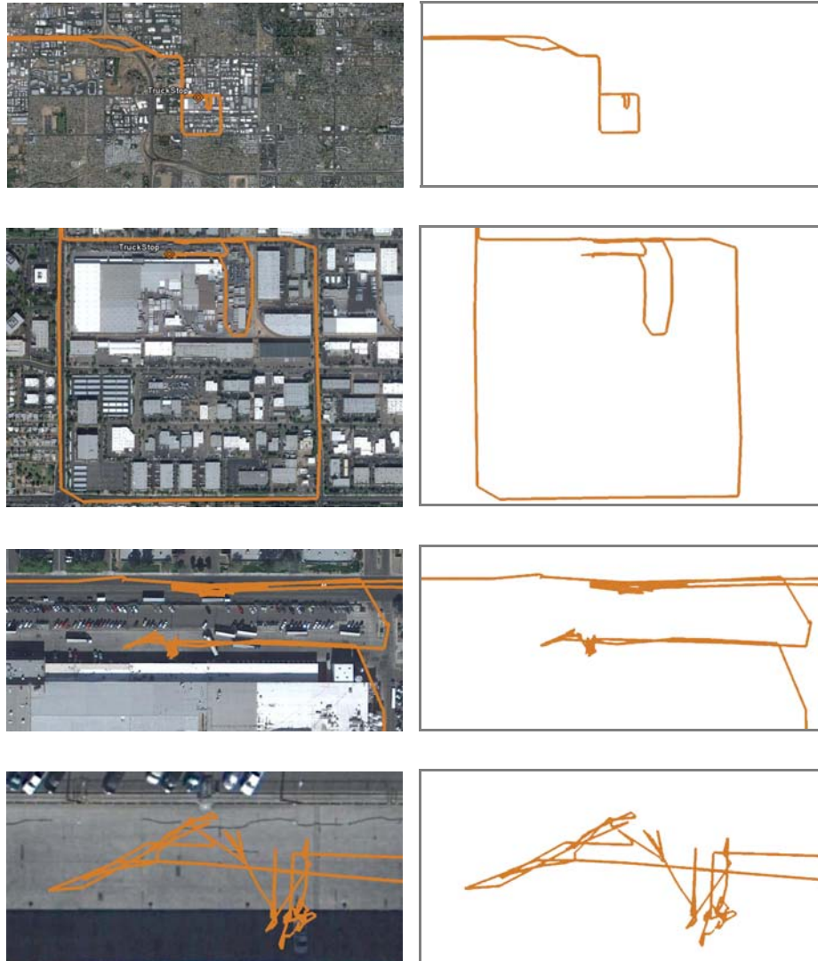
Fig. 6 (continued). The milk plant shown in Figs. 6a-d is displayed here by Google Earth. The driver's efforts for precise parking before loading/unloading can be clearly perceived. The trajectory sections are repeated in the right images without the satellite images (e-l).
