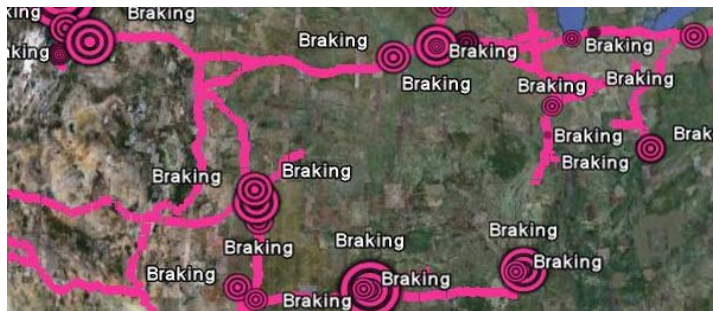
Fig. 3. Truck routes with braking locations as displayed by Google Earth. The marker size represents the strength of the intended braking.
