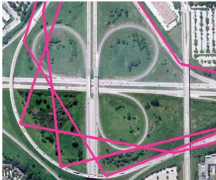
Fig. 4. Off-the-road artifacts appear in the visualization – due to the low spatial sampling frequency used for the route – at a curving road section of a motorway junction.
