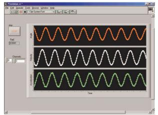
**FIGURE 2.** Combination of a pendulum with coaxial rotary potentiometer. The curves on the front panel of the virtual instrument show the angular position, velocity and acceleration (from top to bottom, respectively).
