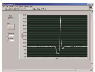
**FIGURE 7.** Combination of az acceleration sensor chip and a long bar. The virtual instrument has measured the acceleration during free fall and the quick deceleration thereafter.
