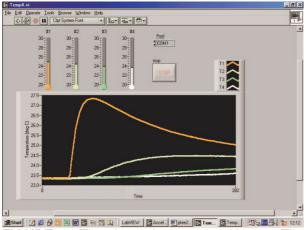
**FIGURE 8.** The thermal wave experiment. The four curves correspond to the temperatures at the four equidistant points.
