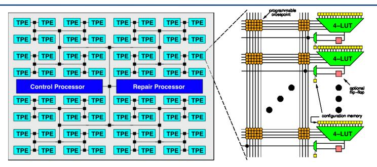
980 Task Processing Elements (TPE) each comparable to Pentium IV 11nm geometry Control and Repair processor 140nm geometry are highly reliable
