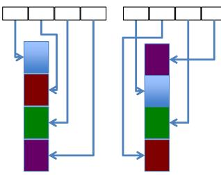
Code and/or data blocks are periodically repositioned in memory so that attacker has to work harder to find a target.
