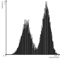
Figure 1: Histogram of a noisy image's  $\mathbf{v}$  component.
