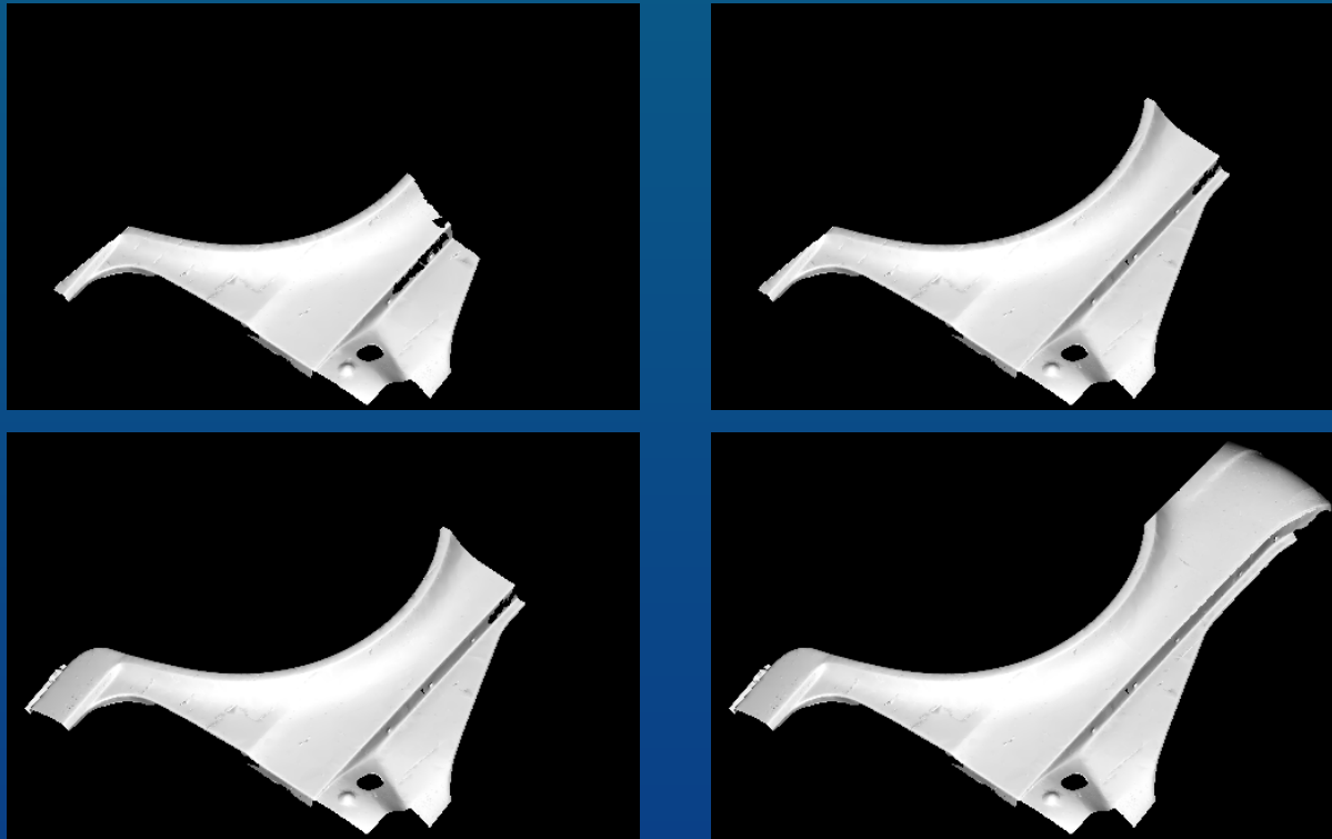
Aligning four measurements of Fiat part . (overlap \approx 20%.)
