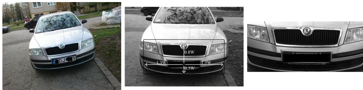
Number plate detection, rotation compensation, ROI extraction
