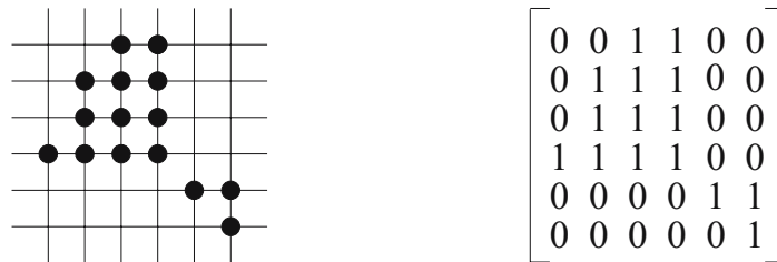
Fig. 1. An hv-convex 8- but not 4-connected discrete set represented by its elements (left) and by a binary matrix (right)
