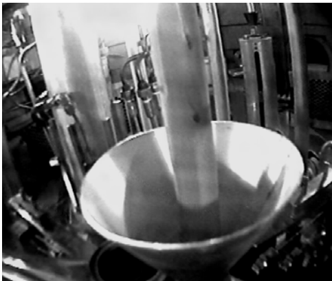
FIGURE 1. Photo of the damaged K5 control rod. FIGURE 2. Photo of the crack on the surface of the damaged K5 control rod
