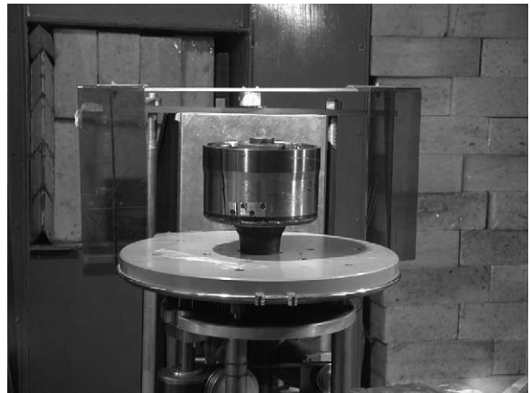
Fig. 3. VISCO clutch on the rotating table used in the tomographic experiments.
