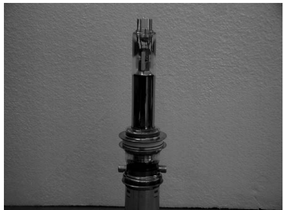
Fig. 4. The Vidicon tube.
