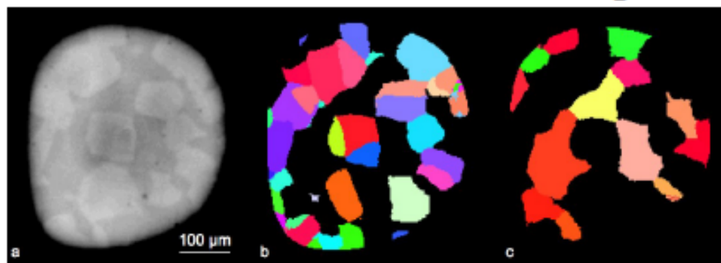
a) Phase Contrast Tomography b) DCT – Austenite c) DCT – Ferrite
