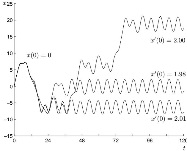
Figure 2: Some trajectories of the forced damped pendulum.
