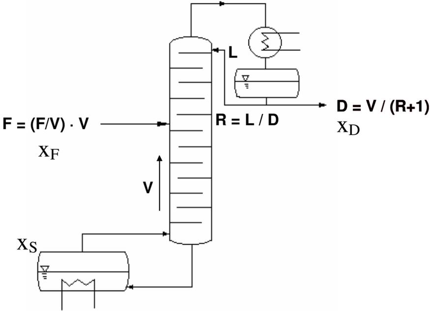
Figure 1. BED in a rectifier
