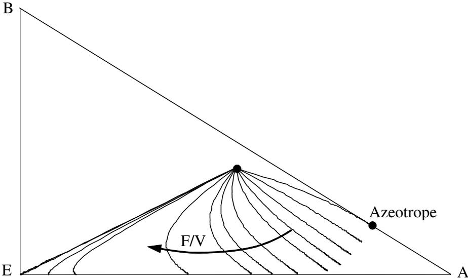
Figure 2. The path of the stable node SN can be determined by computing extractive profiles started from the same single point.
