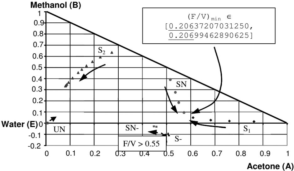
Figure 7. Singular point paths with evolving  $F/V$  at  $R=4$
