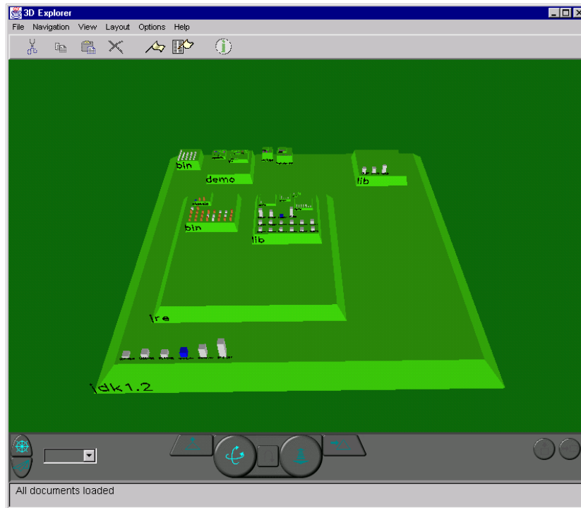
Figure 3.15: An Information Pyramids visualisation of the JDK 1.2 tree. The view from above gives a graphical disk usage. The dashboard provides user navigation. This version uses OpenGL for 3d output.
