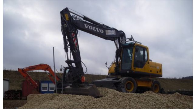
Fig. 7: The autonomous mobile bucket excavator THOR
