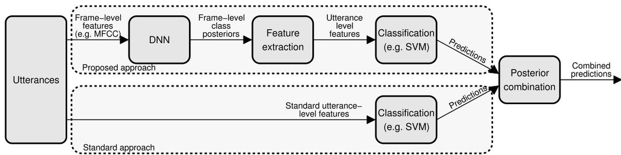
Fig. 1. The workflow of the proposed paralinguistic processing scheme.
