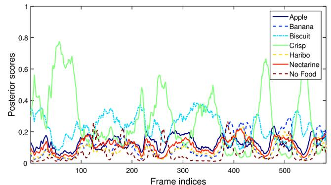
Fig. 2. The frame-level posterior scores obtained for an utterance of the Eating Condition corpus; the correct class for this example is ‘Crisp’.
