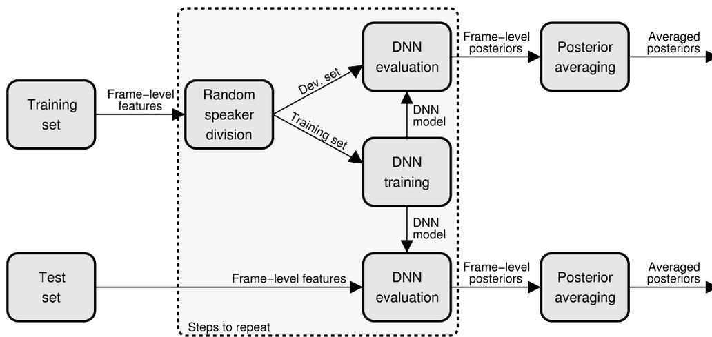
Fig. 3. The workflow of the proposed method for obtaining frame-level posterior estimates.
