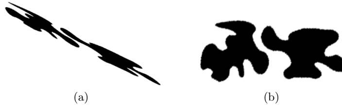
Fig. 4. Registration result. (a) Distorted observation of the sample image in Fig. 1 (rotated, scaled and sheared). (b) Registration result of the proposed method. The image is obtained by applying the recovered inverse transformation to the observation . The registration error was \delta = 0.95\% and \epsilon = 1.59 pixel.
