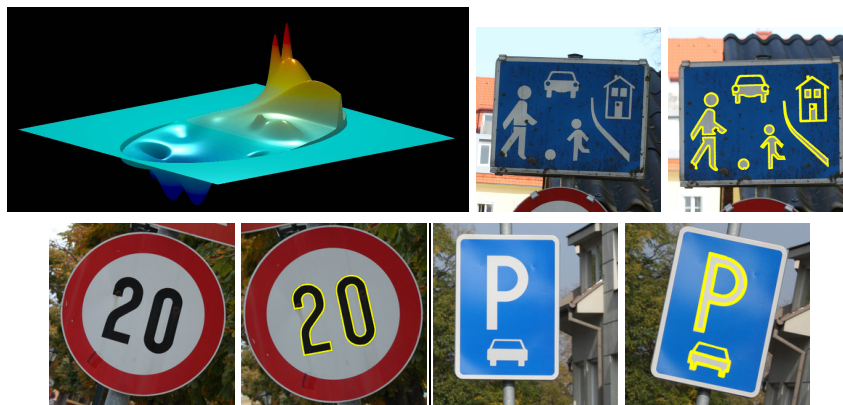
Fig. 3. Alignment of a traffic sign images using a linear system of equations with multiple shape parts. The first image shows the elliptic integration domain with the compound covariant function fitted over the template . Registration results are shown as an overlaid contour on the second image.
