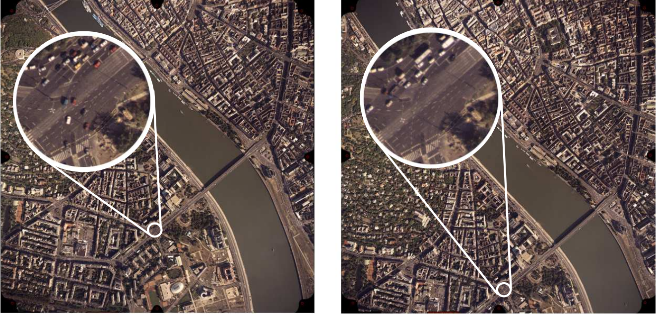
Fig. 1. High resolution stereo image pair taken by the Hungarian Ministry of Defence Mapping Company © above Budapest with a few sec. time difference.
