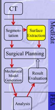
1. Use the Segmented volume and create a triangle mesh of the surface
