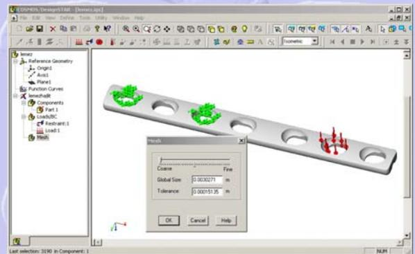
Generation of the finite element mesh
