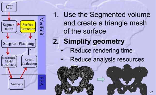
1. Use the Segmented volume and create a triangle mesh of the surface
