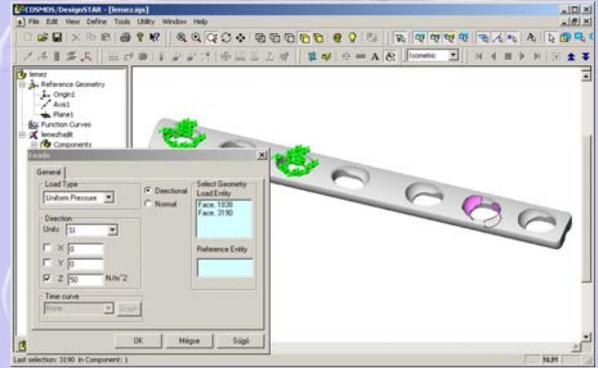
Load type, direction, and loaded area is defined
