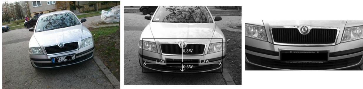
Number plate detection, rotation compensation, ROI extraction
