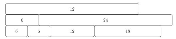
First we schedule 6 onto the fastest machine, its load being 6/3 = 2 then, then the second 6 goes on the second machine, its load becoming 6/2 = 3, then the third job of size 6 goes again to the third machine, its load becoming 4, then the 12 goes again to the third machine, its load becoming 8 (on machine 2 the load would be 9 while it would be 12 on the first), and so on, the makespan is now 15.
