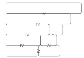
It is easy to see that this schedule is the one produced by the LPT algorithm: clearly, LPT distributes the first m (largest) jobs to the machines, one job for each machine, then the last n-m jobs fill the machines "bottom-up". Thus, if  $p_n > L^*/3$ , then LPT produces an optimal solution, so L cannot be larger than  $\frac{4}{3}L^*$  is this case either.
