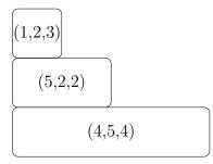
If now we get the job (4, 2, 1), then the load of machine 1 would increase to 5, the load of machine 2 would increase to 4, and the load of machine 3 would increase to 5. Since 3 is the least amongst these possibilities, we schedule (4, 2, 1) onto machine 2. (Observe that this is not the machine which could finish the job in the least time.)
