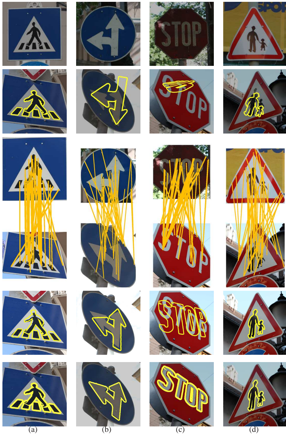
Figure 6.5: Registration results on traffic signs. The templates are in the first row, then the results obtained by SIFT [142]+homest [141] (second row), where the images show point correspondences between the images found by SIFT [142] in the third row. The results obtained by Shape Context [60]+homest [141] (fourth row) and the proposed method in the last row. The contours of the registered images are overlaid.
