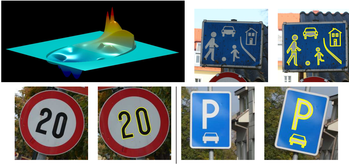
Figure 5.7: Alignment of a traffic sign images using a linear system of equations with multiple shape parts. The first image shows the elliptic integration domain with the compound covariant function fitted over the template. Registration results are shown as an overlaid contour on the second image.
