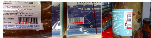
Figure 28. Localization results on real images of products with various distortions.
