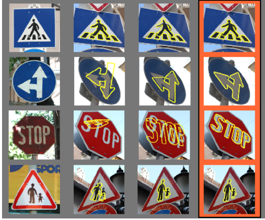
Figure 20. Registration of traffic sign images using a plane projective deformation model. The first column shows the templates , while the second, third, and fourth columns show the registration result as an overlaid yellow contour for SIFT, Shape Context, and our method, respectively.
