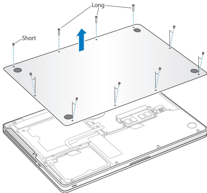
**Important:** When you remove the bottom case, you expose sensitive internal components. Avoid touching anything other than the hard drive assembly when you remove or add a hard disk drive.
