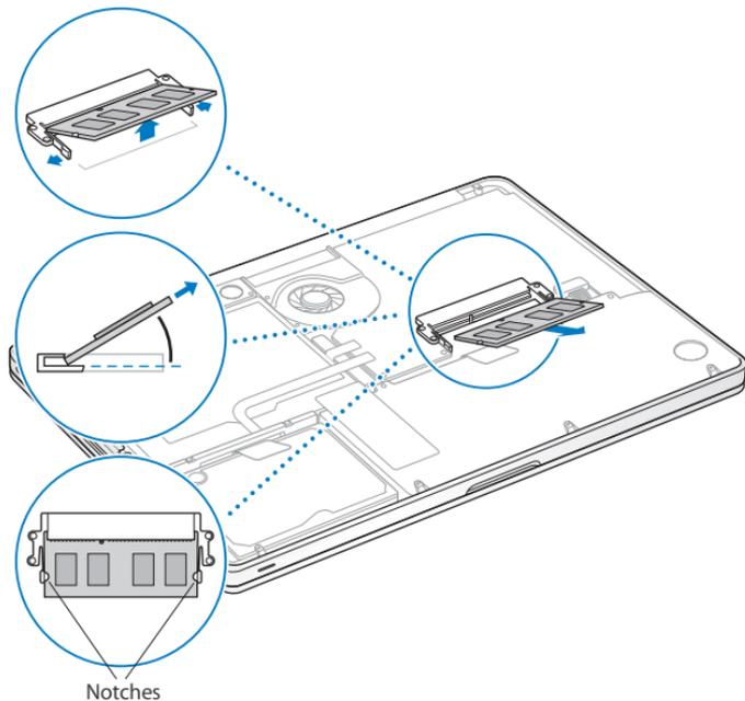
3 Hold the memory module by its notches and remove it from the slot.
