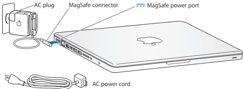
To extend the reach of your power adapter, replace the AC plug with the AC power cord. First pull the AC plug up to remove it from the adapter, and then attach the included AC power cord to the adapter, making sure it's seated firmly.
