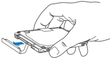
The connector is attached to a cable and remains in the hard disk drive bay.
