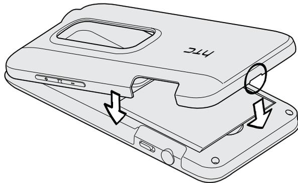
2. Press the sides and the top part of the back cover down to lock the cover into place. You'll hear clicks when the small tabs underneath the back cover are locked in place.
