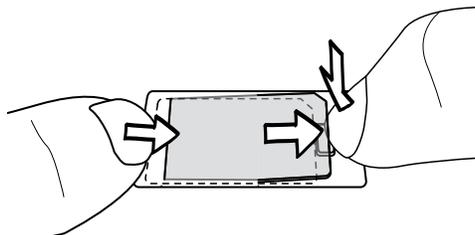
4. Slide the SIM card out from the SIM card slot.
