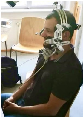
Figure 3: A person has been recorded his speech and tongue movements by the Ultrasound Tongue Imaging device.
