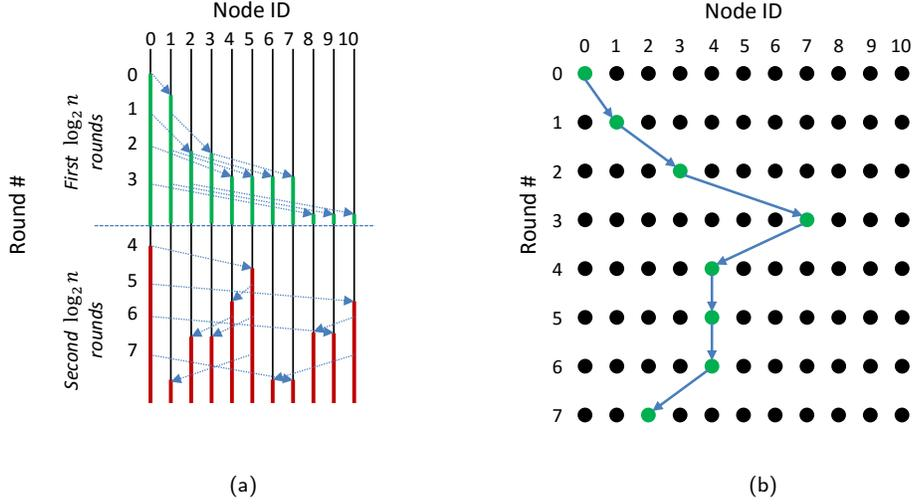
Fig. 1. (a) Information flow from node 0 in our scheme, showing two full epidemic cycles of  $\log_2 n$  rounds each. Every process sends and receives one message per round; we omitted the extra messages to reduce clutter. Similarly, although each round can be viewed as a new epidemic, the figure just shows two. (b) Example of the path taken by a tunneled message, from node 0 to node 3. This message would have 5 layers of onion encryption, since it has 5 different recipients.
