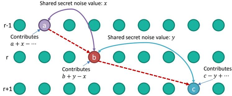
Fig. 3. Example of the paired noise generation scheme. If a query starts on round  $r$  when node  $b$  has predecessor  $a$  and successor  $c$ , it will add a noise value that it shares with  $c$  and subtract a noise value that it shares with  $a$  before contributing its data to the query.
